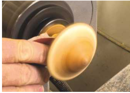
▲ Pic.10 He parts off by carefully supporting the work with one hand while applying the 3mm parting tool; with variable speed slow it down, or you could use a saw
